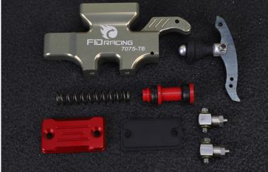
Master pump is made of high strength alloy 7075-T6, CNC machined in high precision and hard-anodized. It is dual Y-ring piston design. Piston shaft is red POM material, with excellent strength and anti-friction property. Others include stainless steel tube connectors, HRC60° 65Mn spring brake pedal, piano-wire return spring.
